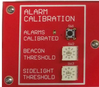
Figure 7 – Alarm Calibration Inputs
